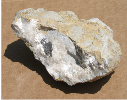
Figure 6.7: The dark mineral embedded in the rock is naturally occurring zinc sulfide.
